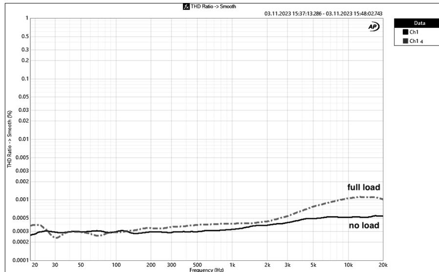
Figure 7: Austrian Audio *Full Score one* | THD vs frequency | 90 kHz bandwidth
