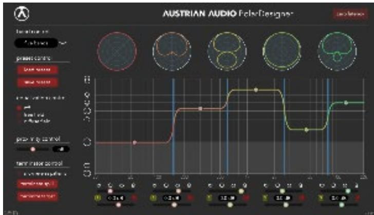
Recording to your DAW using both outputs of the OC818 enables the use of the PolarDesigner™ DAW-Plugin in post production. Craft different polar pattern responses across 1 to 5 crossover bands. Phase Linear and Synch-Channel. Use Terminator Ai for eliminating or rescuing selected frequencies and instruments.
